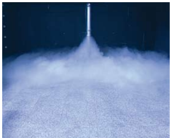
Displacement diffuser type QR-SA -1000 – dia. 400 360° open V_{supply} = 700 \text{ m}^3/\text{h} \Delta T = -4\text{K}
