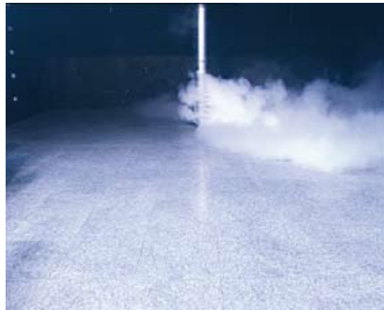
Displacement diffuser type QR-SA -1000 – dia. 400 180° open V_{supply} = 700 \text{ m}^3/\text{h} \Delta T = -4\text{K}
