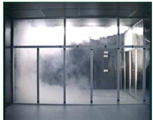
Combined suppl and extraction outlet KWVB-S in a smoke test Length 1000 mm, V_{\text{supply/extr.}} 100 \text{ m}^3/\text{h} \Delta T = -6\text{K}
