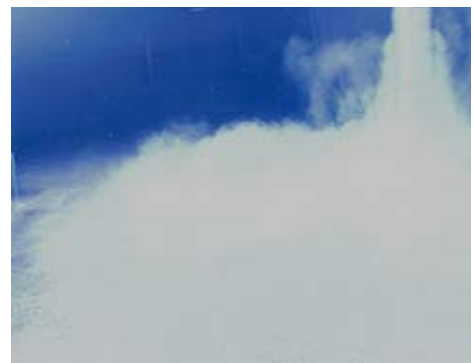
Displacement diffuser type QR-KH - 2000 dia. 580 for cooling applications V_{supply} = 5000 \text{ m}^3/\text{h} \Delta T = -5K
